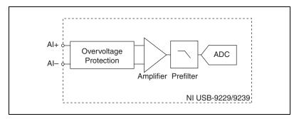
Figure 10. Input Circuitry for One Channel
